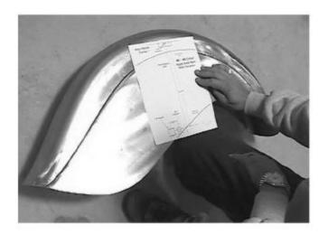
Lay the template over the right side of the fender. The Top and bottom fender lines and the pre-scribed square hole will position the template as needed.
